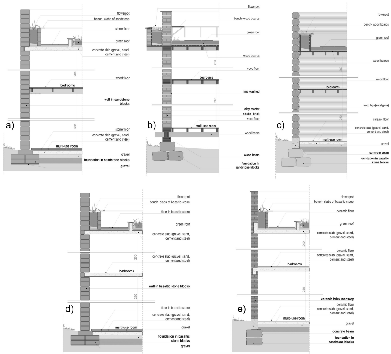
Figure 3: Subsystems sections. a) sandstone; b) enxaimel; c) eucalyptus wood logs; d) basalt stone; e) clay fired ceramic brick
